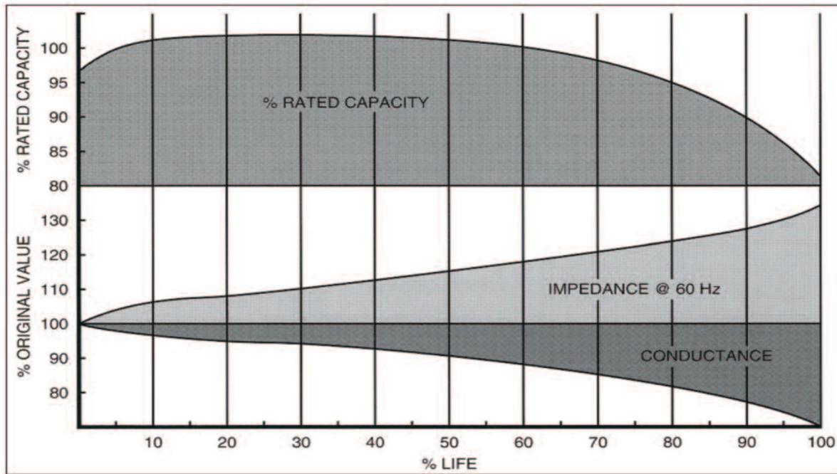
Figure 4 - VRLA Battery Impedance and Conductance Vs. Capacity and Age
