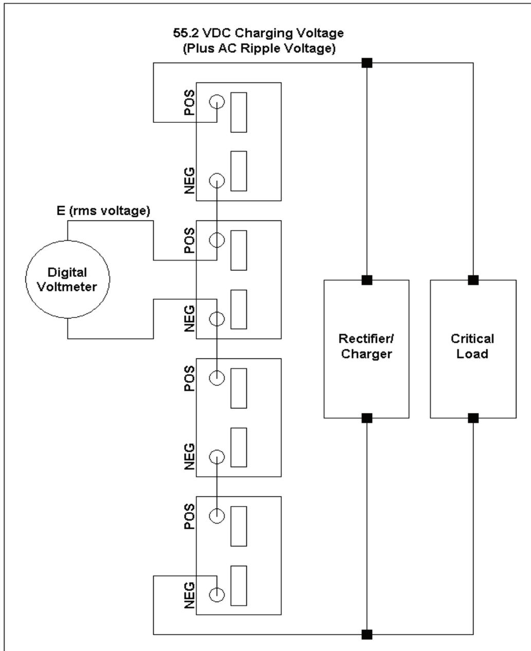
Figure 5 - VRLA Battery Impedance (Ripple Voltage) Measurement
