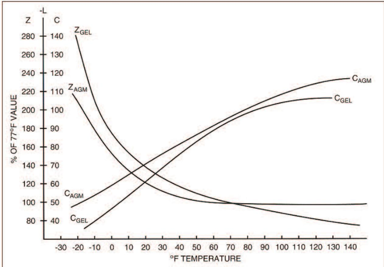
Figure 6-Impedance and Conductance VS. Temperature
