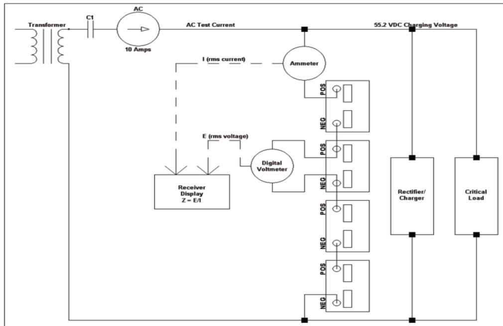
Figure 3 - VRLA Battery Impedance Test Setup
